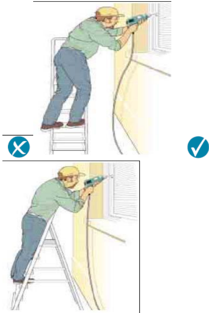
Incorrect – steps side on to work activity
